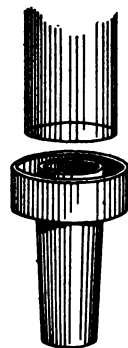
Fig. 5. Cast-iron tube with collar. One-fourth nat- ural size.
